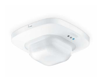
The IR Quattro DCS is a digital passive infrared presence detector setting a new standard in lighting control with minimal movement required for human presence detection. It features a single pyroelectric detector with a high performance lens system creating 1,760 switching zones. Included light level feature provides the option to dim and turn lights off when sufficient daylight is present for additional energy savings.
